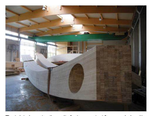
The twisted construction units feature a cutout from a spiral and/or a helix, requiring direct, twisted gluing for which there are few existing examples.
