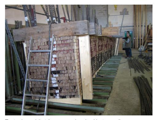
Tests showed that Accoya can be glued just as well as conventional glued-laminated timber when using the specific resorcinol resin.
