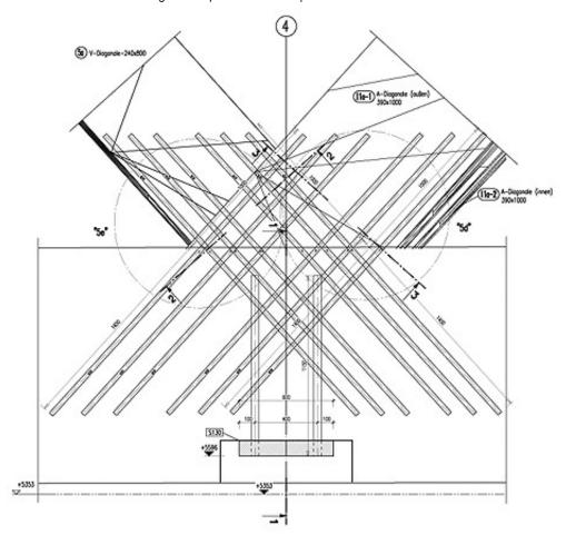
Glued thread rods were used as bending resistant main methods of jointing. The bars have partial lengths more than 6 feet, 7 inches, and are drilled into the cross-grained wood of the diagonals.
